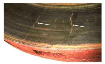
Fig.2. Thermal Craking In Disc Brakes[2]
