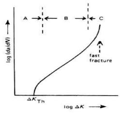
Fig.4 Crack Growth Curve For A Fatigue Loading [3]
